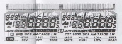
LCD Segmentation Circuit Diagram
