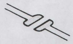
☐ Hold the chip with tweezers in the desired position, and apply the soldering iron with a motion line as indicated by the arrow in the diagram below. Do not apply heat for more than 3 seconds.
